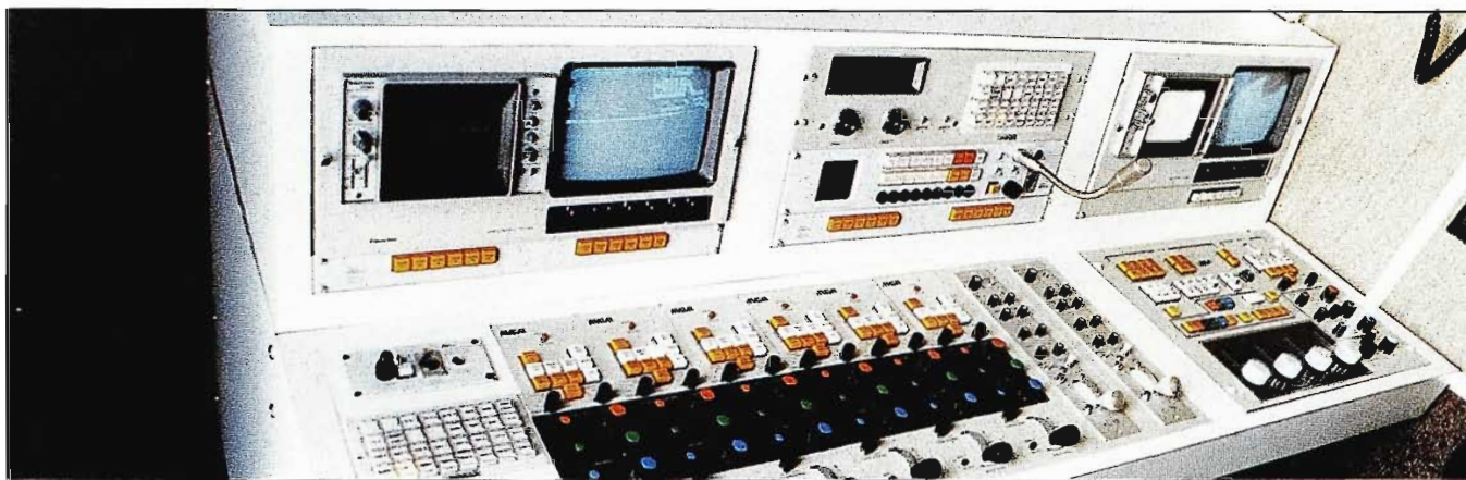
Video control for TK-47 automatic cameras is a compact facility with console for set-up terminal and RCUs for individual cameras.
