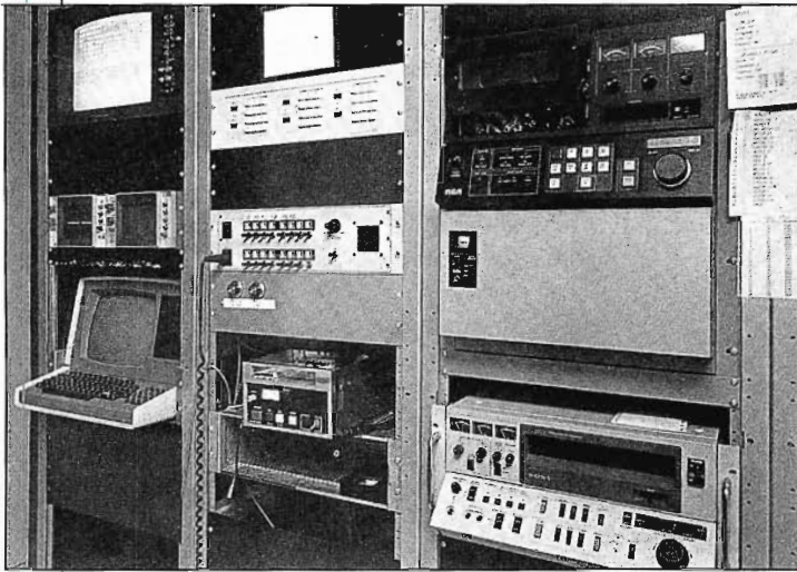
Control center for the Multi-cassette playback system includes an Encoder/Keyboard Unit and a Master Record HR-2 ChromaTrak 1/2-inch studio VTR.
