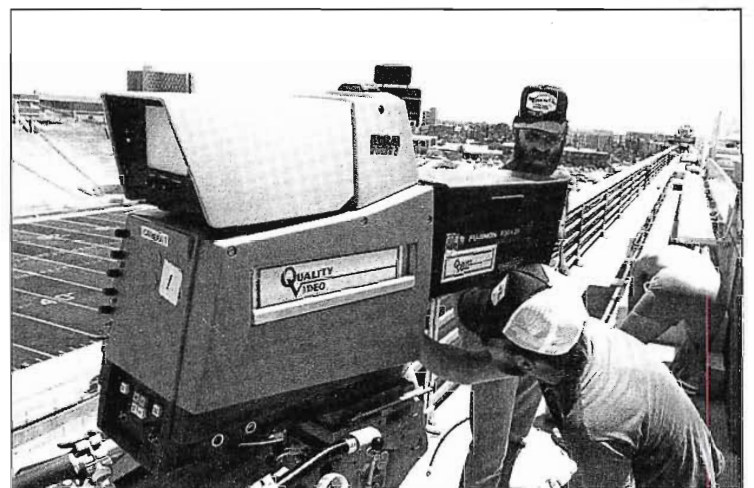
Quick set-up is essential for QVLV operations. Automatic computer set-up and checks for TK-47 cameras provide optimum performance in minimum time.
