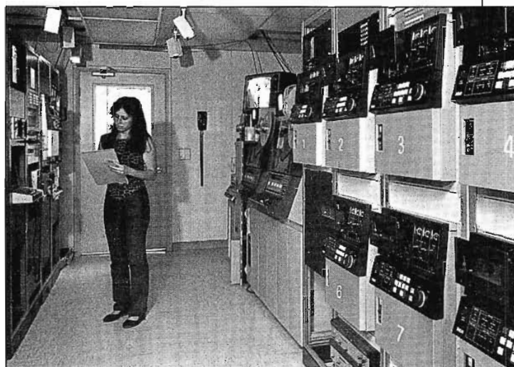
Tape center at TV-39 with "Auto-Cart" system at right and operator at the Encoder/Keyboard unit.
